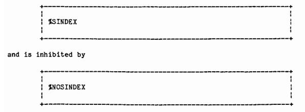
If either of these commands is used, it should appear prior to the first segment. The default setting is "SINDEX".
